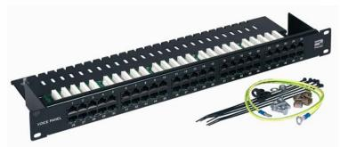
The 50 way voice integration patch panel has six IDC connectors to every 8 way RJ45 socket, this ensures that analogue, digital and ISDN voice systems will have easy migration into structured cabling. This patch panel is ideally suited within the horizontal or backbone cable distribution planes. The perforated cable management system is ideally suited to support the weight of larger multi-paired cables.
